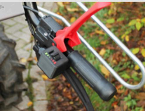
Electrically controlled steering levers with variable zero turn function
