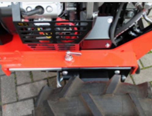
mechanical/hydraulic axle displacement, to balance the unit
